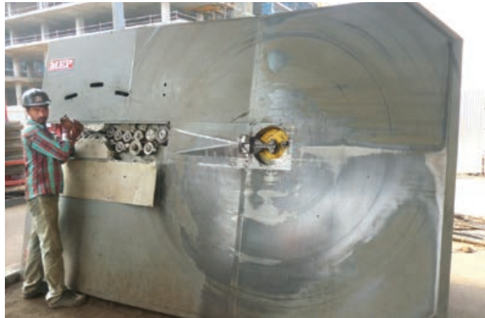
Automatic Rebar Cut and Bend machine
