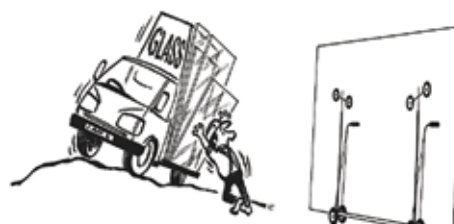
Ensure Vehicle on Even ground
